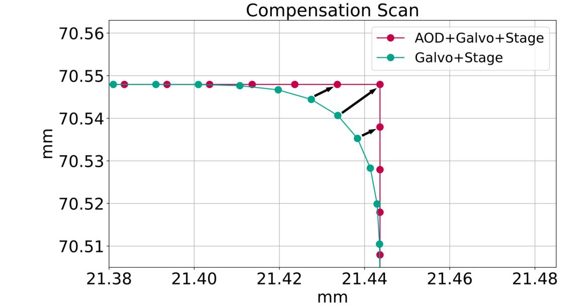
Resulting combined scan with sharp corner geometries.
