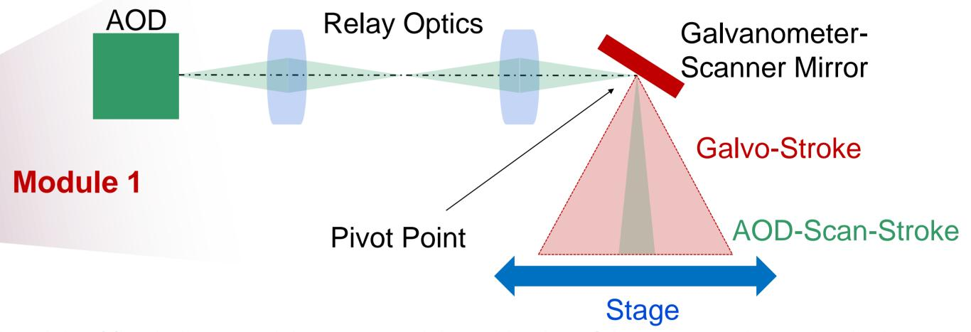
Principle of first built up module: a sequential combination of the two scanning technologies (acousto-optics and galvanometer technology)
